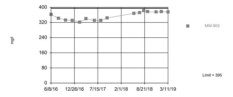
Non-parametric test used in lieu of parametric prediction limit because the Shapiro Francia normality test showed the data to be non-normal at the 0.01 alpha level. Limit is highest of 82 background values. Annual per-constituent alpha = 0.0001433. Individual comparison alpha = 0.0001024 (1 of 3). Assumes 6 future values. Seasonality was not detected with 95% confidence.
